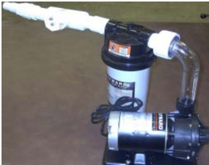
Figure 5.1 Ionizer "T" attaches to filter. Note that the ionizer "T" is oriented slightly above horizontal - about 5 degrees.
